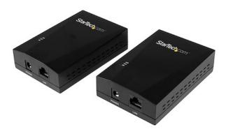
The StarTech.com VDSL2 Ethernet extender kit lets you connect a remote network segment or device to your network, using RJ11 phone cable.
