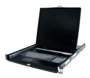
This 1U Rackmount LCD KVM Console provides a complete keyboard, video and mouse control point, integrated neatly into only 1U of rack/cabinet storage space - a space efficient-solution that provides total KVM control right from a server rack.
