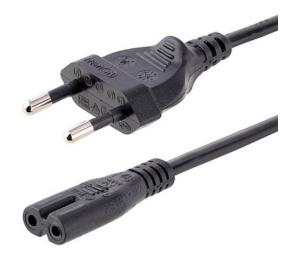
The 752E-2M-POWER-LEAD 2m Laptop Power Cord features one EU plug (CEE 7/16 Alternative II) and one non-polarized IEC 60320 C7 Connector It is a suitable replacement cable for a Lenovo, IBM, or other compatible laptop power bricks that features a C8 inlet.
