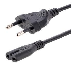
The 752E-3M-POWER-LEAD 3m Laptop Power Cord features one EU plug (CEE 7/16 Alternative II) and one non-polarized IEC 60320 C7 Connector It is a suitable replacement cable for a Lenovo, IBM, or other compatible laptop power bricks that features a C8 inlet.
