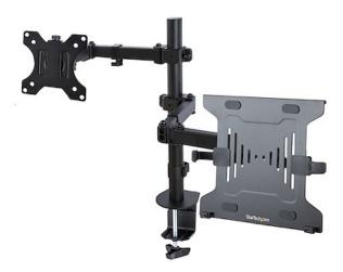
Increase your desk space and add versatility and ergonomics to your work/home setup with this VESA-compatible laptop and monitor desk mount. The laptop tray (11.8x11in / 300x280mm) is large enough to hold a laptop between 9.4-16.5in (240-420mm) wide, 1in (25.4mm) thick, and up to 10lbs (4.5kg). The monitor arm allows you to mount a VESA compatible (75x75mm or 100x100mm) display up to 32in with a maximum weight of 17.6lbs (8kg).
