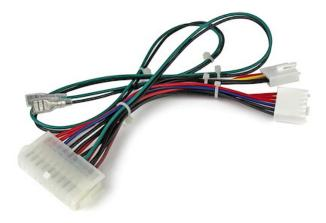
This ATX to AT Motherboard Power Converter Cable adapter allows you to use a standard ATX power supply with an older AT motherboard.
