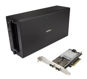
This Thunderbolt 3 to fiber network adapter connects your Thunderbolt 3 enabled device to a 10GbE network. The adapter combines the Thunderbolt 3 technology of TB31PCIEX16 with the 10GbE dual-fiber connection of PEX20000SFPI (Intel 82599 chipset). The assembled adapter features one DisplayPort output, one additional Thunderbolt 3 port, and two open 10GbE SFP+ slots.
