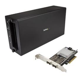
This Thunderbolt 3 to fiber network adapter connects your Thunderbolt 3 enabled device to a 10GbE network. The adapter combines the Thunderbolt 3 technology of TB31PCIEX16 with the 10GbE dual-fiber connection of PEX20000SFPI (Intel 82599 chipset). The assembled adapter features one DisplayPort output, one additional Thunderbolt 3 port, and two open 10GbE SFP+ slots.
