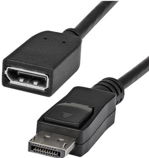
The DPEXT6L 6-foot, DisplayPort Video Extension Cable supports 21.6 Gbps bandwidth, giving a full 4K x 2K (3840 x 2400 at 60Hz) resolution and 3D Stereo display (2560 x 1600 at 120Hz). This DP1.2 cable also provides additional features such as High Bit Rate 2 (HBR2), 8 Audio Channels, Multi-Stream Transport (MST) for connecting multiple displays and Global Time Code (GTC) for sub-micro video/audio sync.
