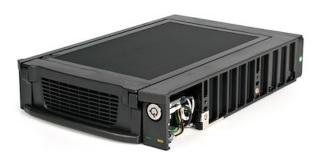
This high quality Removable ATA Hard Drive Drawer/Mobile Rack delivers a convenient storage solution, allowing you to quickly swap ATA66/ATA100 and ATA133 hard drives in and out of a computer without having to open the computer case.
