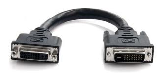
The DVIEXTAA6IN 6-inch DVI-I Port Saver Cable/coupler avoids expensive repairs to a computer or display. It does this by extending the port by 6in, thereby eliminating the weight and stress that would typically be placed on the port by a DVI cable. This is especially useful in an environment where cables are unplugged and re-inserted frequently.
