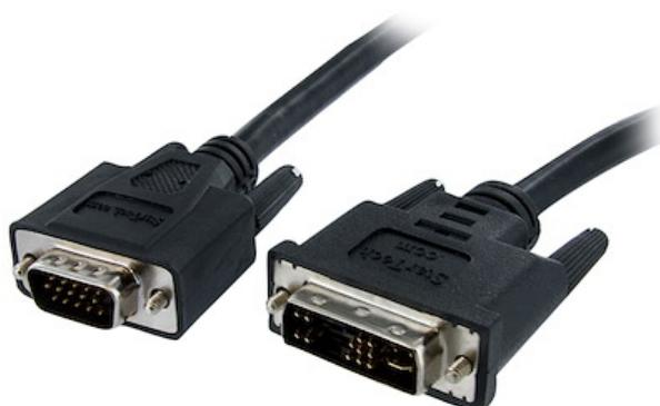
The DVIVGAMM6 6-foot DVI to VGA Monitor Cable features a DVI (analog) male connector and a VGA (High Density D-Sub) male connector, providing a cost-effective way to connect an analog or a dual mode Flat Panel Display to a PC or Mac® computer with a DVI Analog Video Card.
