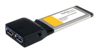
The ECUSB3S22 2-Port ExpressCard USB 3.2 Gen 1 Card adds 2 SuperSpeed USB 3.2 Gen 1 ports to an ExpressCard-enabled computer system, using a 34mm form factor that will fit in both 34mm and 54mm slots, along with ports mounted side-by-side for easy access.
