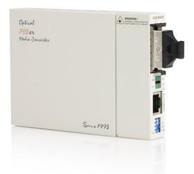
This Gigabit Ethernet to MM Fiber Media Converter creates a cost-effective Gigabit Ethernet-fiber link, transparently converting to/from 1000BaseT Ethernet signals and 1000BaseSX optical signals to extend an Ethernet network connection over a multimode fiber backbone.
