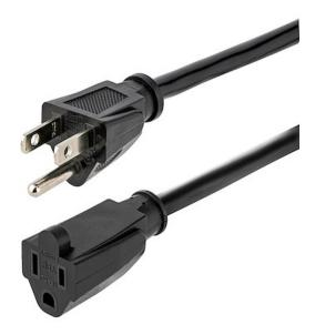
The HX-15F-POWER-CORD is a NEMA 5-15P to NEMA 5-15R power extension cable which features heavy gauge wire (14 AWG) that is suitable for handling 125V at 15A, making it a reliable solution for connecting larger servers to PDUs (Power Distribution Units).
