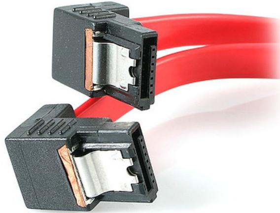
The LSATA18RA2 Right Angle (90-degree) SATA Cable enables you to plug in your SATA hard drive in hard to reach areas or tight spaces, using right-angled SATA connectors to reduce the amount of space required at the connection point and supports full SATA 3.0 bandwidth of up to 6Gbps when used with SATA 3.0 compliant drives.
