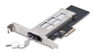
Utilize an available PCle 4.0 x4 expansion slot for the installation, removal, or interchange of PCle M.2 SSDs. The drive tray accommodates M-Key M.2 NVMe SSDs in 2230, 2242, 2260, and 2280 sizes.
