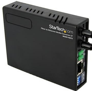
This Ethernet to MM Fiber Media Converter creates a cost-effective Ethernet to fiber link, transparently converting to/from 10Base-T or 100Base-Tx Ethernet signals and 100Base-Fx optical signals to extend an Ethernet network connection over a multimode fiber backbone.
