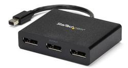
This MST hub lets you connect three DisplayPort monitors to your Mini DisplayPort computer. MST works on any Windows device that supports DisplayPort 1.2, such as models of the Lenovo Think Pad and Microsoft Surface. When connected to earlier revisions of DisplayPort, such as DP 1.1 the MST hub acts as a video splitter.
