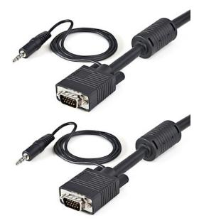
The MXTHQMM15MA 15-meter High Resolution VGA Cable with Audio is a high quality SVGA cable designed to provide the highest video quality possible through VGA - a single cable solution for connecting both video between a VGA video card and monitor, and audio connections between a sound card and external audio device.
