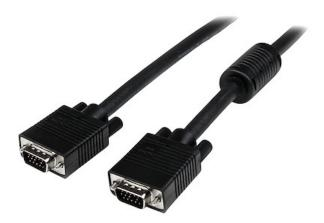
This 18in High Resolution VGA Monitor Cable is designed to provide the highest video quality possible through VGA. Ideally suited for high resolution VGA applications (1024x768 and above), this high quality coaxial VGA cable eliminates picture "ghosting" and fuzzy images inherent to non-coaxial cables, and provides superior EMI interference protection by using ferrite cores near the connector ends.
