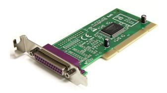
The PCI1P\_LP 1 Port Low Profile PCI Parallel Adapter Card adds one IEEE 1284 port to your small form factor PC, with data transfer speeds of up to 1.5 Mbps – up to 3 times faster than on-board parallel ports. The adapter card features a low profile design that is suited to small form factor computer cases, while including a full height bracket to adapt to any installation.
