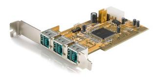
The PCI312PUSB 3 Port PCI 12V PoweredUSB Adapter Card adds three Powered USB (USB PlusPower) ports to any computer, through an available PCI Slot.
