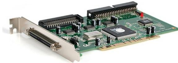
This PCI based Ultra Wide SCSI Controller Adapter card lets you control up to 15 Wide SCSI devices, supporting high speed single-ended SCSI bus transfer rates of up to 40MBps, and is equipped with a dedicated on-board processor to ensure optimized performance.
