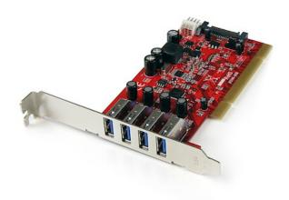
The PCIUSB3S4 4-Port PCI to USB 3.2 Gen 1 Card enables legacy PCI slots to support the SuperSpeed USB 3.2 Gen 1 standard, which is capable of data transfer rates up to 5 Gbps. Using USB 3.2 Gen 1 devices with this card will increase data transfer rates with up to 1.3 Gbps of available bandwidth (PCI bus limit) - more than doubling performance compared to a USB 2.0 connection. Note: Some newer PCs may use a PCIe to PCI bridge which can cause unexpected compatibility issues with this product.
