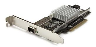
This fiber network card delivers reliable, high-performance network connectivity, by adding an open SFP+ slot to your server or high-powered workstation. It provides an easy and cost-effective way to upgrade your server or workstation to a 10 Gigabit fiber network using the SFP+ module of your choice and gives you the flexibility to use either multimode or single-mode fiber.
