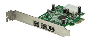
This 3 Port PCI Express FireWire adapter card can be installed in a PCI Express slot to add two IEEE1394b (FireWire 800 - 9 pin) ports and one IEEE1394a (FireWire 400 - 6 pin) port, providing broad compatibility with a wide range of FireWire devices (e.g. DV camcorders, external hard drives, digital cameras, etc.).
