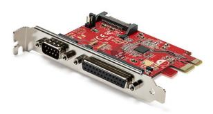
This PCIe Parallel and Serial Combo Card installs into a single PCI-Express x1 slot in your computer, and adds a DB25 IEEE 1284 parallel port and DB9 RS 232 serial port to your system. The PEX1S1P950 is the latest version of our popular PEX1S1P952 combo card.
