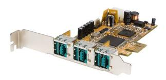
The PEX312PUSB 3 Port PCI Express 12V PoweredUSB Adapter Card allows you to add three Powered USB (USB PlusPower) ports to any standard form-factor computer, using an available PCI Express Slot.
