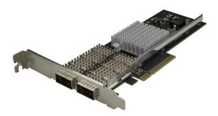
Get fast, high-bandwidth connectivity with this dual-port QSFP+ Network Interface Card. It adds two open QSFP+ slots to your server or workstation. The 40G NIC features an Intel controller and provides redundant network links with reliable performance. It's ideal for high-demand database servers, virtualized servers and agile data centers that require infrastructure updates with no downtime.
