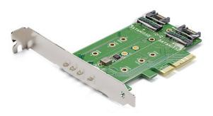
This 3-port M.2 SSD adapter card is one of the only cards that supports both PCIe and SATA-based M.2 SSDs (solid-state drives). It's a versatile way to expand the overall storage capacity of your desktop PC or server. Plus, because it supports a high-speed PCIe M.2 drive, you can increase the speed and performance of your computer.
