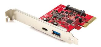
This USB 3.1 card helps prepare you for the next generation of USB connectivity and performance. Now you can access USB 3.1 Gen 2 devices at 10Gbps, which is twice the speed of traditional USB 3.0 devices. (USB 3.0 is also known as USB 3.1 Gen 1.)
