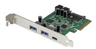
This 5-port USB 3.1 combo card makes it easy to add to the performance and connectivity of your computer. It's one of the only USB 3.1 cards to offer a USB Type-C port (10Gbps), traditional USB Type-A ports (5Gbps), and a motherboard header.
