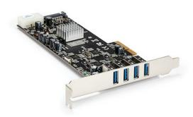
The PEXUSB3S44V 4-Port PCI Express USB 3.2 Gen 1 Card lets you add four, dedicated 5 Gbps USB 3.2 Gen 1 ports to your PCIe x4-enabled PC. This independent port architecture improves USB 3.2 Gen 1 performance by transferring data on four individual channels to your computer, giving you faster file transfers.
