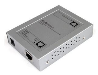
The POEINJ100 10/100 Mbps PoE Power over Ethernet Injector with 48V Output converts standard 90-260V/AC power into low-voltage DC power that can run over existing Cat5 (or better) network cable to power IEEE 802.3at compliant network accessories.
