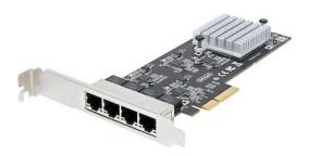
This quad-port 2.5 GbE network interface card (NIC) features an Intel I225-V chipset with Intel vPro technology, to enhance performance and data integrity across four 2.5G ethernet connections. The variable multispeed options (2.5/1Gbps and 100/10Mbps) enable support for both new and legacy network hardware. Utilize existing Cat5e or CAT6 cabling infrastructure while adding NBASE-T (802.3bz) compatibility for seamless integration.
