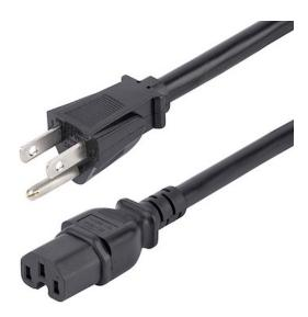
The PXT515C158 8-foot Computer Power Cord features a C15 connector rated for high-temperature equipment, as well as 14 AWG wire suitable for high power connections - a reliable solution for connecting to NEMA 5-15P Power Distribution Units (PDU) located in switchgear rooms and data center environments, or large server applications that require a higher rated, heavier gauge cable.
