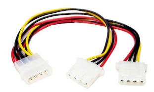
The PYO2L LP4 to 2x LP4 Power Y Splitter Cable features one LP4 male connector that breaks out into two LP4 female connectors, providing a cost-effective solution for connecting two LP4 peripheral devices (CD/DVD-ROM drives, IDE hard drives etc.) to a single LP4 connector provided by the computer power supply.
