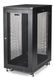
This server rack provides 24Uof storage space in a sleek, secure cabinet for storing standard 19" rack-mount devices such as Dell, HP and IBM servers, along with telecommunication and A/V equipment. The rack is compatible with EIA-310 compliant equipment and supports a total load capacity of 450 kg (992 lb.).
