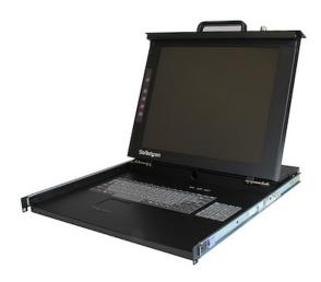
The RKCONS1701GB 1U 17" Rack Mount LCD Console provides a complete keyboard, video and mouse control point, integrated neatly into only 1U of rack/cabinet space - providing complete KVM control right from a server rack.
