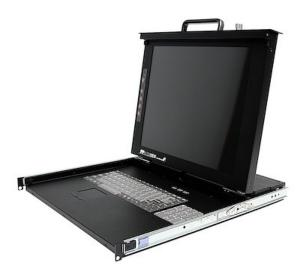
This 1U Rack Mount LCD KVM Console features an integrated 8 Port Multi-Platform KVM Switch module, 17in active matrix LCD monitor, full 106-key keyboard and mouse touchpad neatly combined into 1U of space in any standard rack or cabinet 30in (or greater) in depth.
