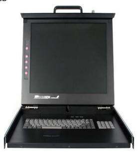
This 1U Rack Mount LCD KVM Console features an integrated 16 Port Multi-Platform KVM Switch module, 19in active matrix LCD monitor, full 106-key keyboard and mouse touchpad neatly combined into 1U of space in any standard rack or cabinet 30in (or greater) in depth.
