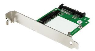
The SAT32MSATPEX mSATA to SATA adapter enables you to connect a mSATA SSD to a standard SATA port, and mount the drive into any desktop expansion slot.
