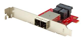
This Mini-SAS adapter lets you convert two internal SFF-8643 ports on a controller card into two external SFF-8644 ports. This enables you to connect external SAS or SATA drives in devices such as a Direct Attached Storage (DAS) device to an internal backplane or SAS controller for additional storage.
