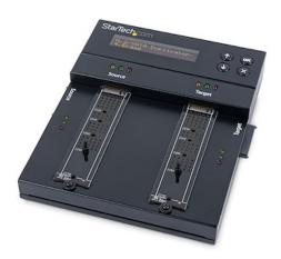
This flexible 1-to-1 drive duplicator and eraser provides a standalone solution for cloning and sanitizing hard drives (HDD) and solid state drives (SSD) without computers or software. The drive duplicator/sanitizer can clone drives at up to 7.5GB per minute, and supports a wide variety of drive types:
