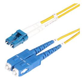
OS2 LC to SC Single Mode Duplex Fiber Optic Patch cable facilitates connectivity across 10G networks. It supports Coarse Wavelength Division Multiplexing (CWDM) across an extended wavelength range of 1260-1625nm, improving channel isolation for optimal signal strength over long distances.
