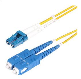
OS2 LC to SC Single Mode Duplex Fiber Optic Patch cable facilitates connectivity across 10G networks. It supports Coarse Wavelength Division Multiplexing (CWDM) across an extended wavelength range of 1260-1625nm, improving channel isolation for optimal signal strength over long distances.
