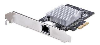
Install this single-port 10GbE PCI Express (PCIe) Network Interface Card (NIC) into a server or computer to enable faster network speeds and enhanced network functionality. This card supports six speeds: 10/5/2.5/1Gbps and 100/10Mbps. The variable speeds permit access to legacy hardware. Alternatively, the 10GBASE-T and NBASE-T capabilities ensure compatibility with the latest network switches and network access points manufactured by Cisco, HPE, and Juniper.
