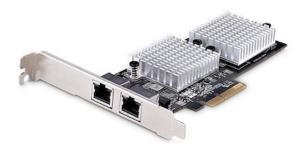
Install this 2-port 10GbE PCI Express (PCIe) Network Interface Card (NIC) with independent controllers into a server or computer to enable fast network speeds and enhanced network functionality by providing failover and redundancy protection to mission-critical servers/applications.
