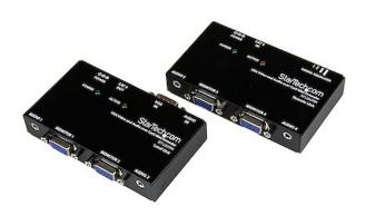
The ST122UTPAEU VGA Video Extender over Cat 5 with Audio allows up to 4 (2 local and 2 remote) monitors to be connected to a single PC. The video signal and corresponding audio are sent to the remote unit over standard 4 pair Category 5 or better (Cat 5e recommended) UTP cable, supporting extended video distances of up to 150m / 500ft.
