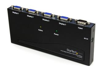
The ST124PROGB 4 Port High Resolution VGA Video Splitter - 350 MHz splits a VGA video source signal to 4 monitors or projectors simultaneously - a professional grade solution that is perfect for presentations, classrooms, tradeshows, or in-store displays, where the highest quality video on several monitors is needed.
